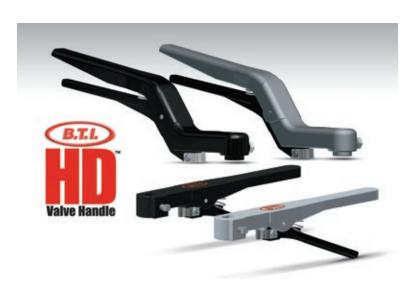
this problem with the newest version of their HD Handle. Replacing the trigger with a composite trigger they have stopped the corrosion build up between the trigger and the stainless steel pivot pin. This offers effortless operation while opening and closing the valve.
