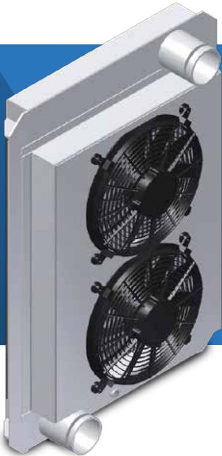
The Bulk Tank Inc. Trailer Mounted Air-to-Air Cooler was developed and designed for pneumatic dry bulk tank trailers in the transport of heat-sensitive products such as sugar, plastic pellets, and resins. In the pneumatic unloading process, compressed air is the conveying medium. When air is compressed it generates heat. The higher the pressure the greater the temperature and temperatures up to 350°F, in a typical operation, can be hazardous to the product load.
